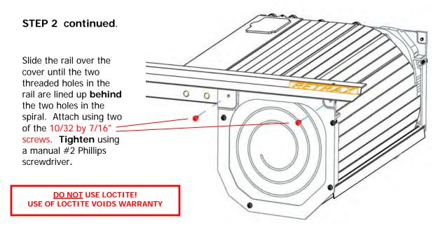
**STEP 3 Install the drivers rail.** Pull the cover out of the canister 6"-8" (See PwertraxONE Installation Supplement on how to move electric cover). Caution: DO NOT allow cover to roll back into canister until rail is installed. Repeat Step #2 to install the driver's rail. Be sure all rail mounting screws are tight.
